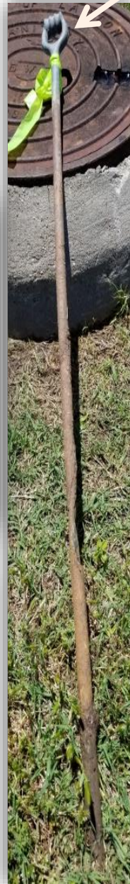
Electric utility's helix anchors
