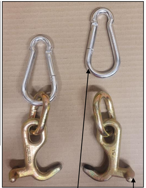
Quick release connector with 2,000 pound working load limit. Manhole lifting hooks have 5,000 pound working load limit.
