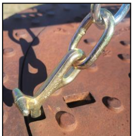
Quick release connector with 2,000 pound working load limit. Manhole lifting hooks have 5,000 pound working load limit.
